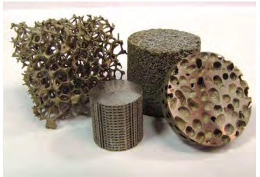
Examples of porous titanium alloy structures made using (from left to right) sacrificial polyurethane foam templates, 3D laser printing, and spaceholder methods.
